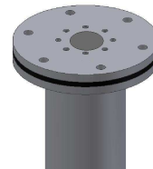
Fit the top flange
